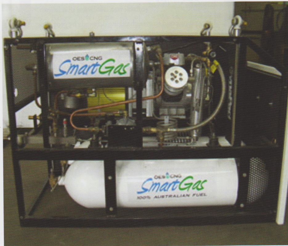
OES says its compressors have run for over 2000 hours in testing and 1000 continuous hours and are the only ones in the world that can fill a car in three minutes..
